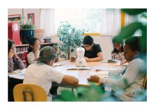
Standing 30cm tall and weighing 1.5kg, AV1 sits neatly on a desk, or can be easily carried by friends in the playground. Two motors enable AV1 to raise and lower its head or revolve up to 360°, enabling the student to see and hear everything going on in the classroom; and 4G and WiFi connectivity ensure it can function both indoors and out. Manchester Hospital School can provide AV1 robots to enable students to continue to access their education as part of our learning pathways.
